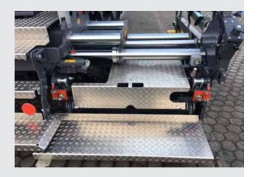
There's no need for supporting rods for the screed, which makes all Dynapac screeds free floating – a must for excellent paving result!
