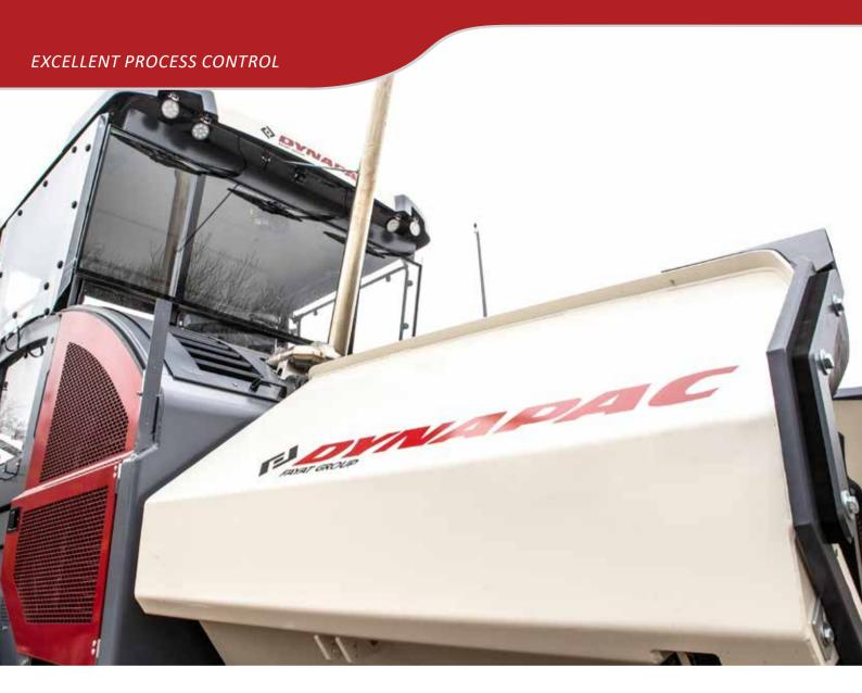
Dynapac SD Pavers are powered by a Cummins QSB6.7 diesel engine with emission Stage IIIA / IV & V. The power unit offers optimized energy conversion through: load-sensitive engine speed control; use of the most efficient pumps and the most compact final drives, incl. motors. The cooling system is driven by a hydraulic motor that is thermostatically controlled for efficient cooling. The CAN-BUS system ensures high operational reliability and centralised control.
