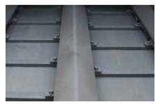
corners prevent cold material being left in the hopper. The conveyor tunnel has been shaped for an optimal flow and minimal segregation. A reversible twin conveyor system, (2 x 580 mm wide), offers smooth transfer. To ensure a flawless material flow, we offer a robust paddle sensor system for proportional control. The new optional hopper front flap re-
