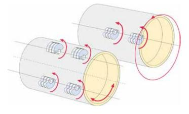
The Dynapac CO4200 has one vibrating drum with two vibration amplitudes and one oscillating drum. This allow the operator to select the system that is most suitable for the application on hand.
