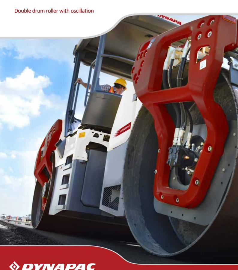
While introducing the large asphalt tandem rollers generation VI, Dynapac also offers the oscillation compaction concept. Meeting the special needs of the oscillation compaction concept, Dynapac has focused on **wear resistance and serviceability** in order to supply a long lasting and user friendly solution.
