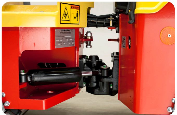
Articulated steering with a maintenance-free hitch and steering cylinder reduces maintenance.
