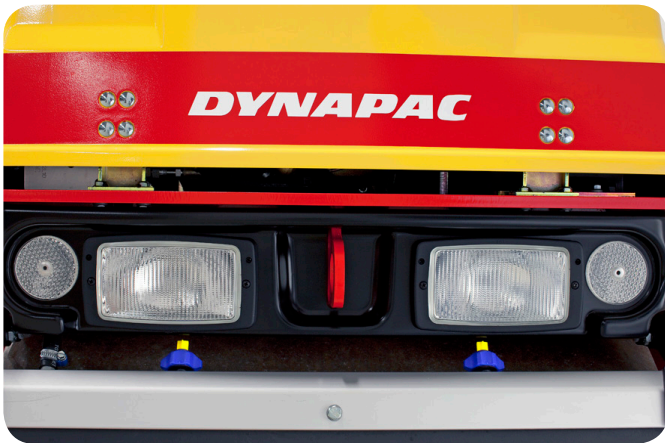
All machines are equipped with a new type of sprinkler tube and nozzles that are self-draining to minimize the risk of ice plugs in cold weather.
